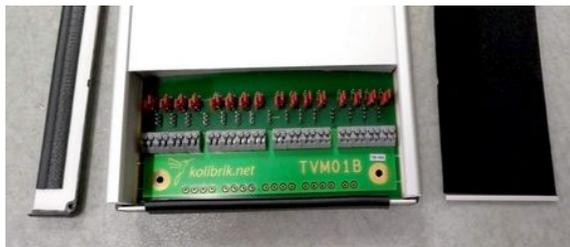
TEVOMET TV16 with removed cover for connection clamps and configuration jumpers
