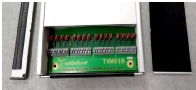
TEVOMET TV16 with removed cover for connection clamps and configuration jumpers
